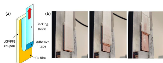
Fig.1: Measurements of adhesion strength of a copper thin film deposited on a polymer. 1
